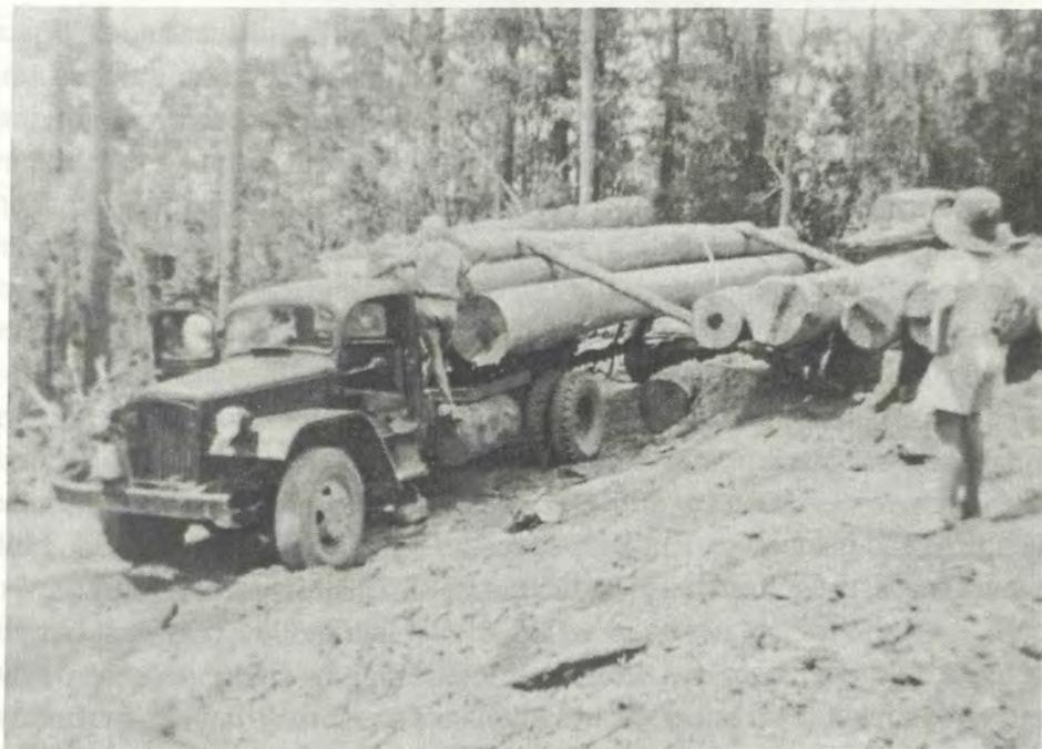
Truck loaded with a number of logs. 1943 model L.H. drive Mack, army release.
