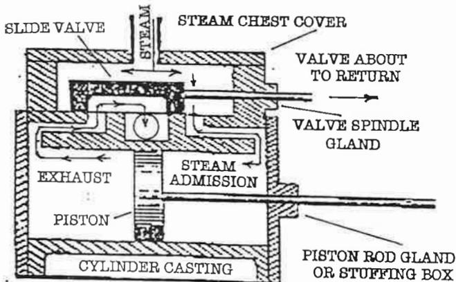
The previous illustrations and explanations show the operation of the slide valve having no lap whatsoever. Although it is common to have no "exhaust lap" in valves used in engines exhausting to atmosphere, "steam lap" (or outside lap) is a definite requirement for the efficient working of all the common types of engines.
