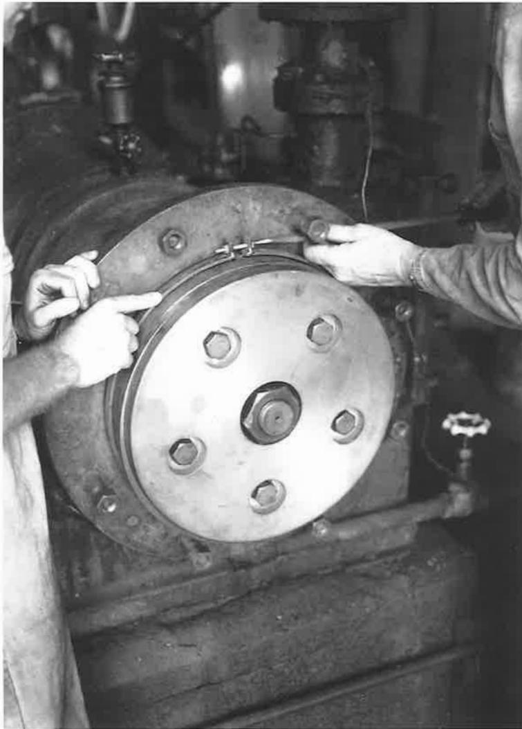
The piston has been entered into the bore and the piston rings are being compressed in order to get them started into the bore also.
