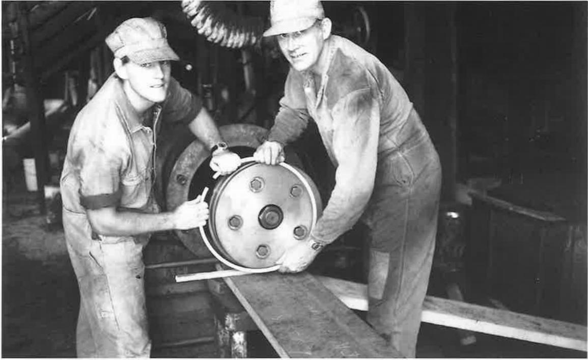
The new piston rings were first checked for "gap clearance" in the bore and then fitted to the piston. John Petersen at left with Alan Johnston.
