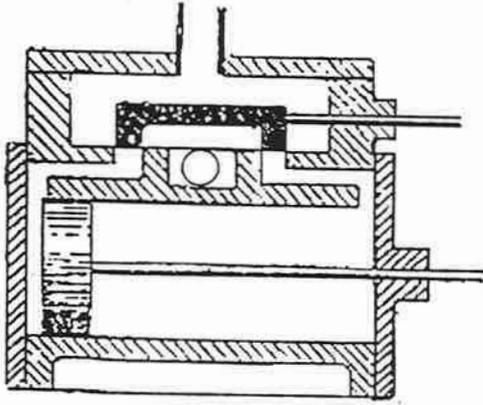
Valve in mid position & about to move to the right which will uncover the left hand port, allowing high pressure steam to enter the left hand end of the cylinder. With the same movement, the right hand port is opened by the exhaust cavity in the underside of the valve, which allows the escape of exhausting steam to the exhaust pipe as the piston moves to the right.
