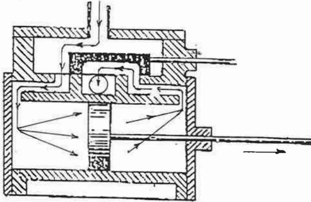
Showing valve at end of its travel and about to return while the piston is shown in mid stroke.
