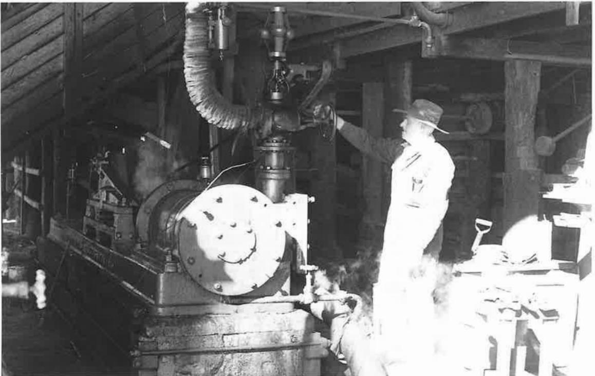
This July 1982 Photo shows Mill Manager Bob Mercer with his right hand on the throttle valve hand wheel situated just below the governor. The asbestos lagged steam pipe can be seen in the middle of the picture coming down from above. The six inch diameter exhaust pipe is to be seen just in front of Bob's legs, with the "outside end" cylinder drain cock line connected in to it.
