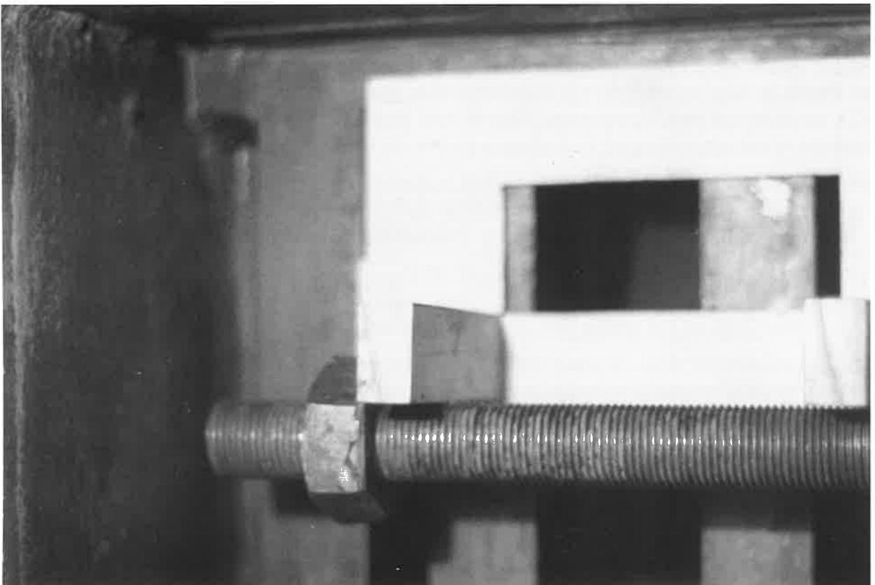
Photo showing close up of the "skeleton valve" in position on the valve spindle and against the port face.
