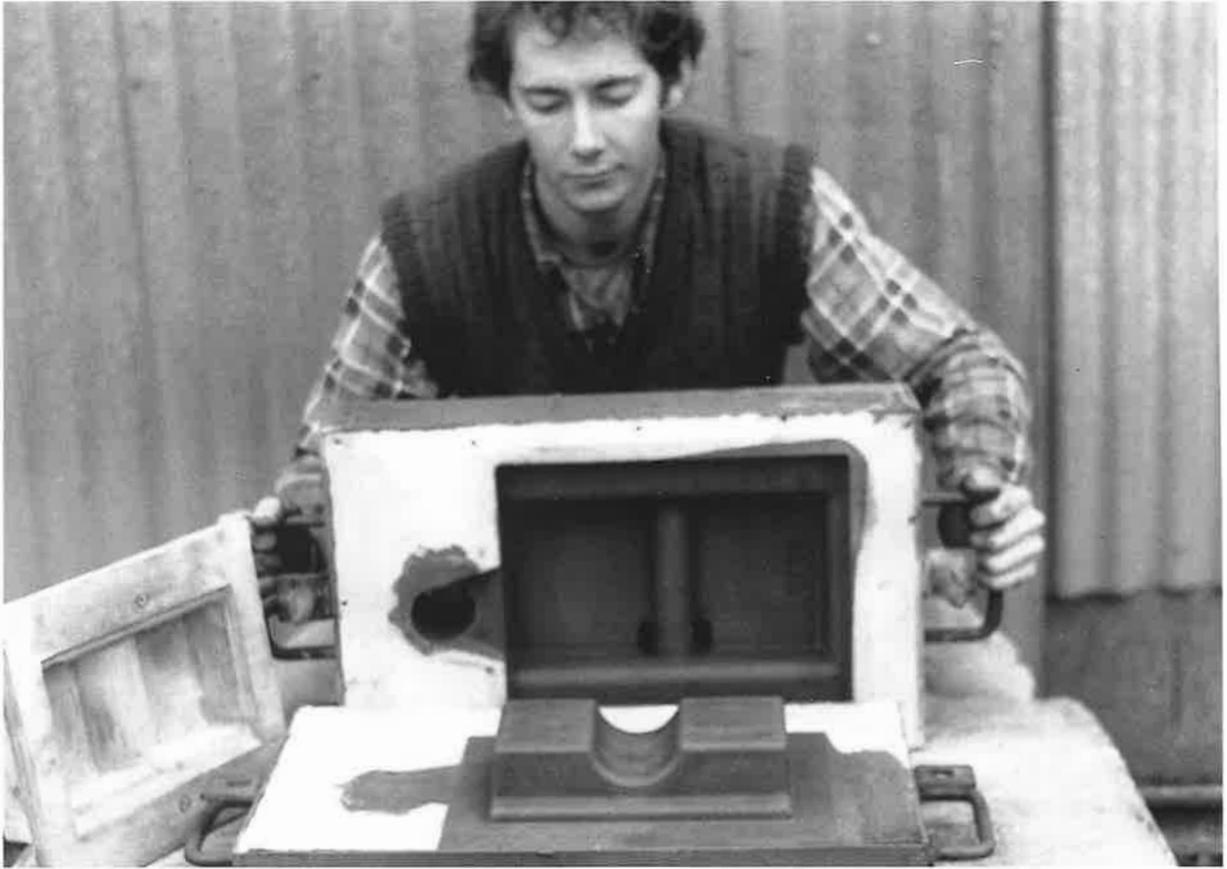
Moulder Neil Anderson is shown about to “close up” the sand mould for the new slide valve ready for casting in molten iron. The pattern which was completed only the night before is shown on the left.
