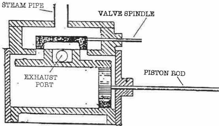
Valve in mid position and moving to the left, allowing high pressure steam to enter the right hand end of the cylinder, thus pushing the piston on its return stroke with the spent exhaust steam escaping through the left hand port.
