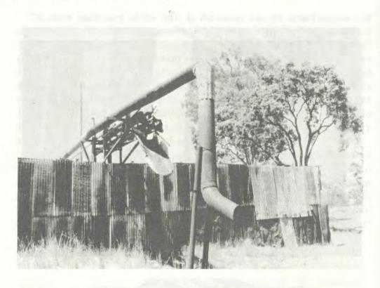
Burning area for waste sawdust and planing shavings. The corrugated iron fence was constructed to prevent sparks from the fire blowing back towards the mill where they would have created a fire danger. Photographed December 1995.
