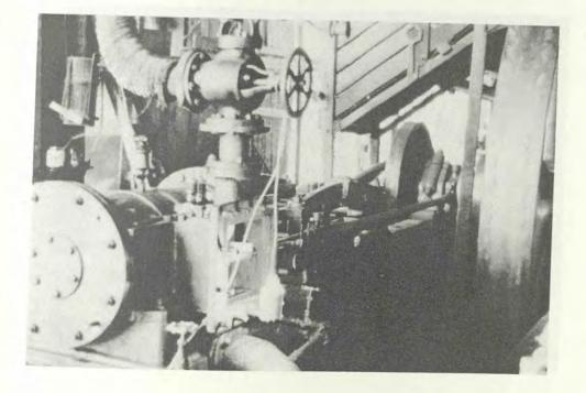
Showing steam chest cover removed and skeleton valve in position. Sawdust chute in background. 1982.
