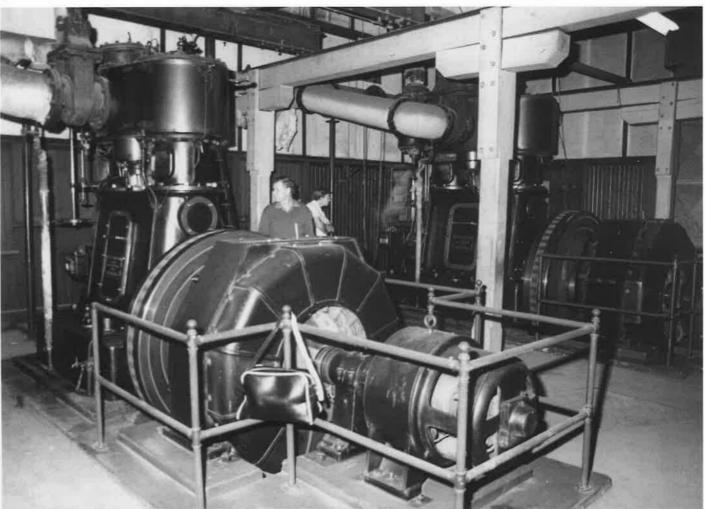
Wilson Hart & Co. Engine Room showing the two Belliss & Morcom Steam Generating Sets installed after the 1934 fire.
