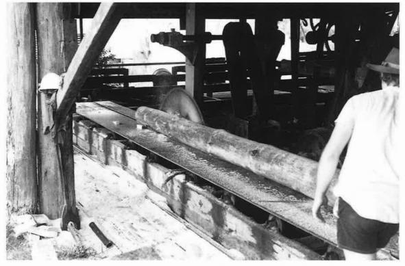
A small Hoop Pine log is fed into the single saw on the Canadian Bench with its long steel travelling table running on rollers. This photograph shows that the saw blade has been removed from the top spindle, it not being necessary when cutting small timber.
