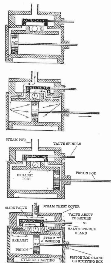
Valve in mid position & about to move to the right which will uncover the left hand port, allowing high pressure steam to enter the left hand end of the cylinder. With the same movement, the right hand port is opened by the exhaust cavity in the underside of the valve, which allows the escape of exhausting steam to the exhaust pipe as the piston moves to the right.
