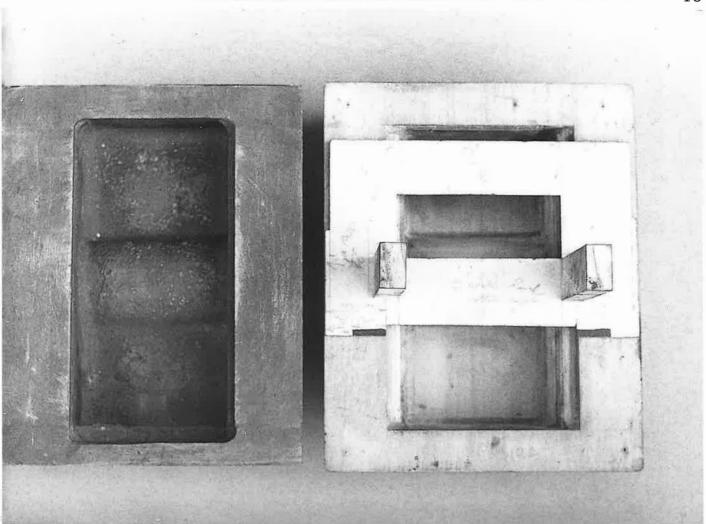
Photograph of the original valve shown on the left, looking at the working face which slides over the "port face" in the steam chest.
