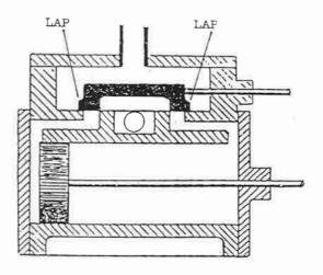
The illustration above shows the slide valve extended on both ends to provide "steam lap". Lap added to the valve causes earlier "cut off" of the admission of steam to the cylinder and effects more economical use of the steam through it being allowed to expand during the power stroke before being exhausted.
