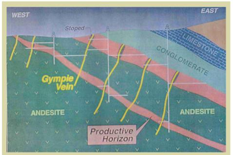
Schematic representation of the dip of the productive beds to the east, showing the resultant deepening of shafts and cross cuts in the exploration for gold bearing reefs. Source: Devex Ltd.
