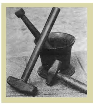
Two Gympie hammers, dolly and dollypot. Invented in Gympie and made by local blacksmiths, Gympie hammers had balanced heads and a small striking area. Their use spread to other mines in Australia and overseas. Source: The Gympie Times, 1991.
