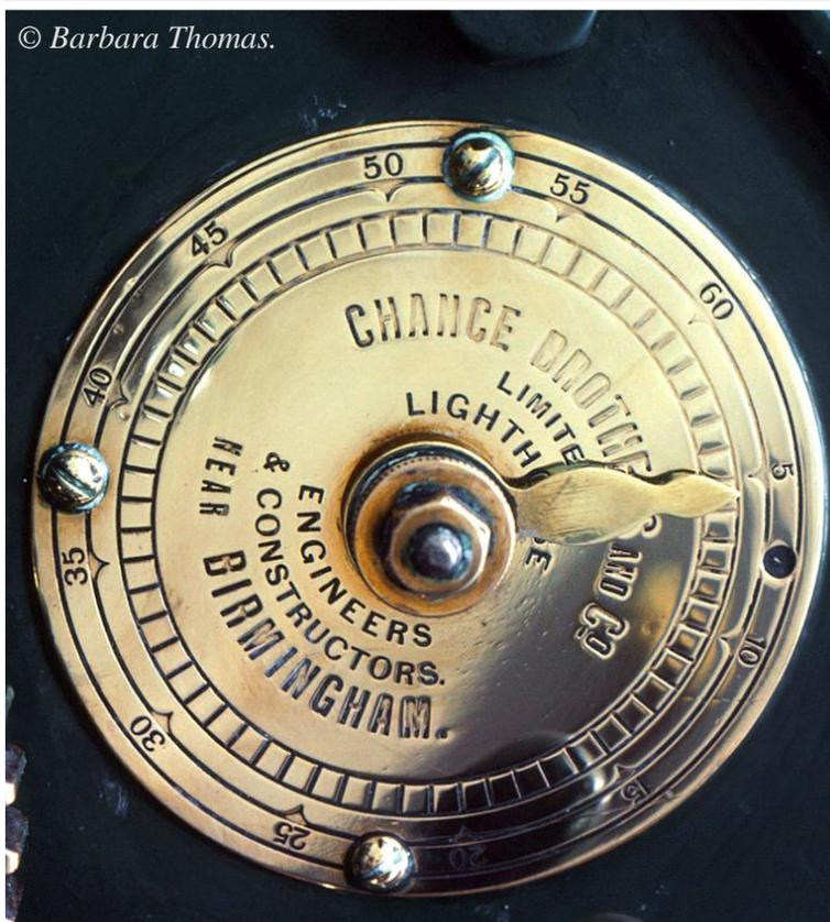
Every two hours the light keeper had to manually wind the weight back up by means of a handle. The centrifugal force developed by two spinning cast iron balls (governors) was used to even out any minor variations caused within the mechanism as the weight descended. The speed of rotation of the balls was adjusted and set by means of the pointer. Note the original 'Chance Brothers' mechanism.
