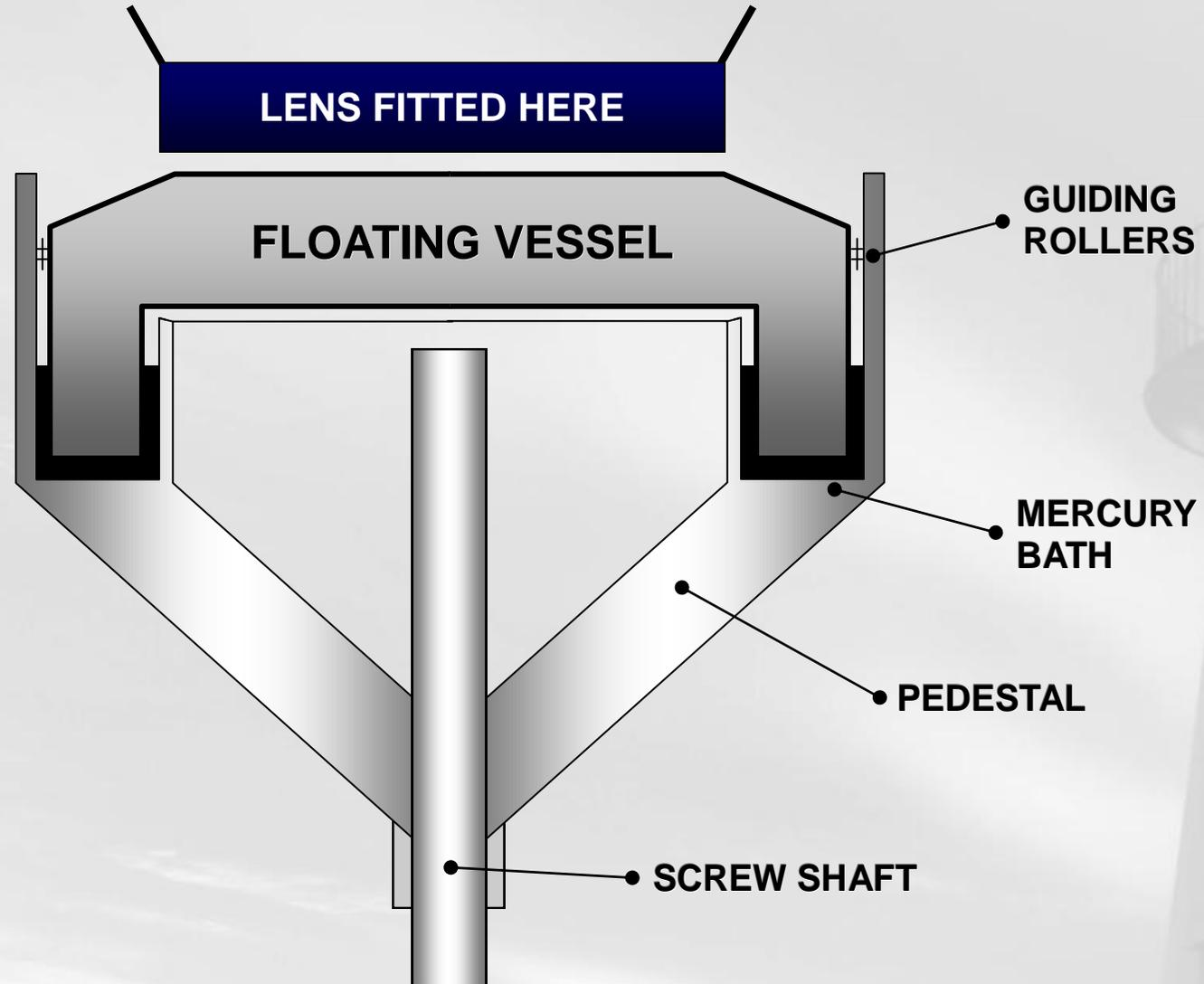
*Mercury was an important part of lighthouse lamp design. When a rotating crystal Fresnel Lens was installed, so was a Mercury Float to enable the heavy lens to rotate easily. As mercury is 13.6 times heavier than water, it was possible to make heavy fixtures to float on it. A first order lens weighed around 4,300 kg and required around 8 litres of mercury to enable it to float.*
