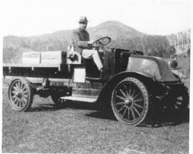
This International truck with solid-rubber tyres and magneto-ignition was used some years later to transport bananas from Seary's Scrub to Seary's Creek. Here it is owned and driven by Mr. Dom Tramacchi.
